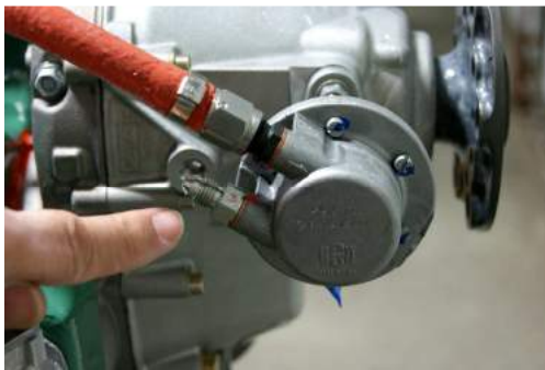
The still common pump, that has no vent. The pump with our the issue has a third Hose-line attachment underneath its body and no external venting system
